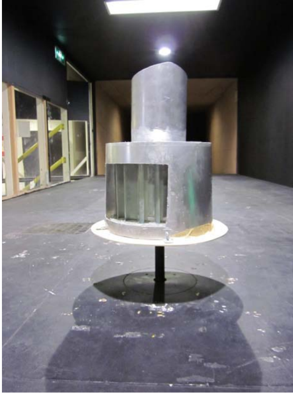
Fig.6: Experimental setup inside the RMIT Industrial Wind Tunnel
